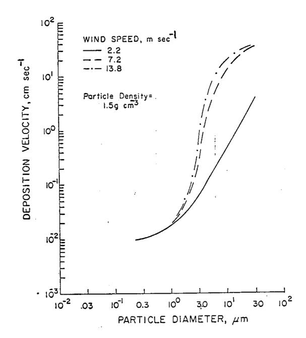
Figure 2. Atmospheric particle deposition velocity to a water surface as a function of particle size and wind speed (After Sehmel and Sutter, 1974)
