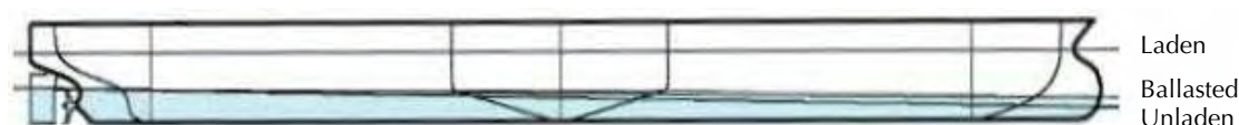
Figure 3-9: NOBS Suezmax tanker design, showing the waterlines in the laden condition and in the typical 'bow-up' unladen and storm ballasted conditions (modified from [6] )
