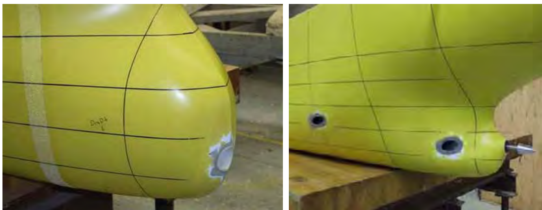
Figure 3-13: Locations of the bow inlet (left) and alternative outlet locations near the stern (right) studied by the University of Michigan project in 2007–08
