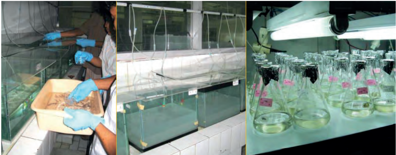
Figure 48 Toxicity testing on mine tailings at Batu Hijau
