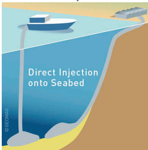
Figure 5.6 Liquid CO 2 placed on the seabed
