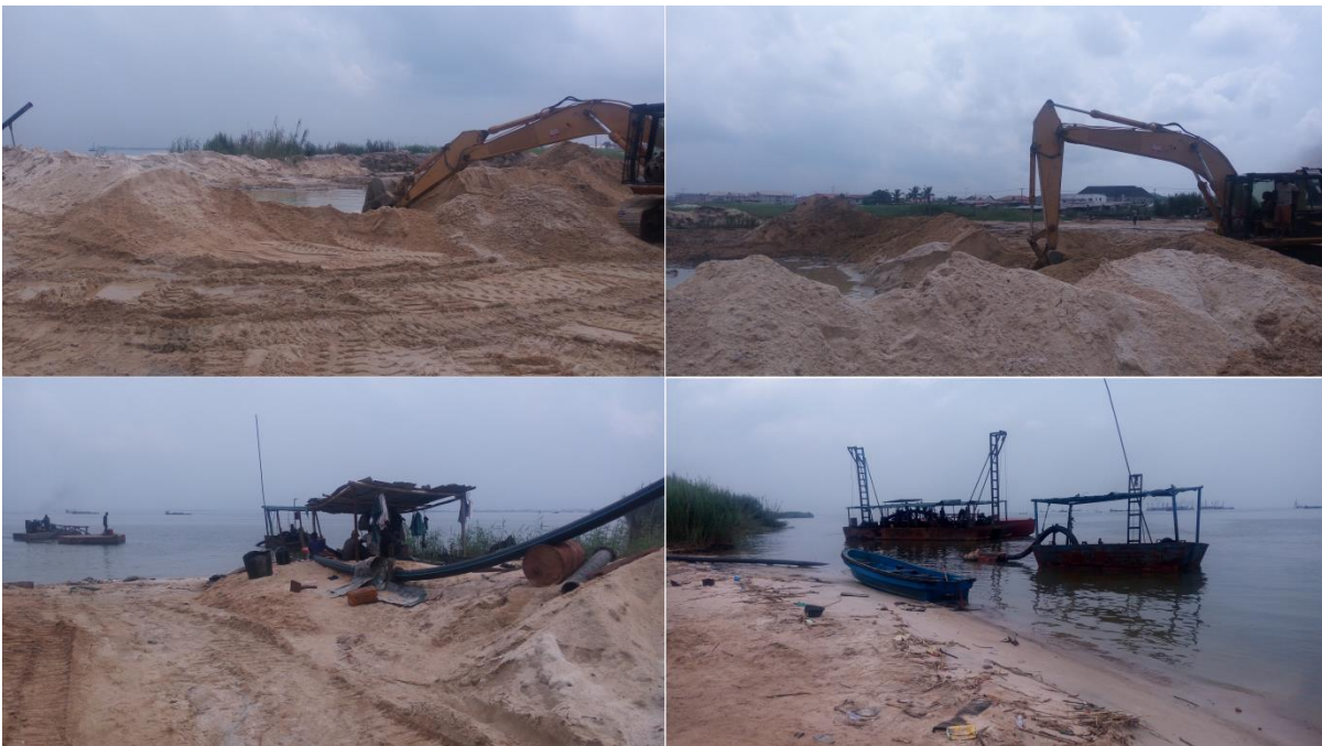
Fig. 1c: Commercial sand mining on the Lagos lagoon in Lagos, Nigeria, (note the dredgers in the foreground) courtesy Bunmi Nubi (NIOMR)
