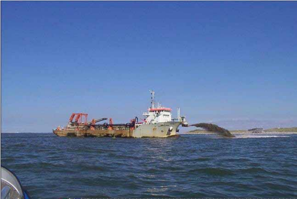
Fig. 2: Industrial sand extraction - typical construction-aggregate trailer suction hopper dredger supplying sand for beach nourishment
