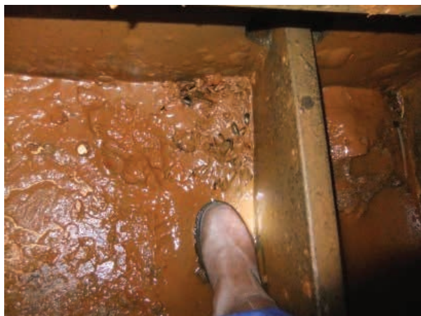
Figure 10 Sediment inside a ballast tank (D. Smith)
