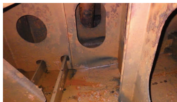
Figure 8 Tank internal structures create many compartments and chambers linked by openings and drain channels (D. Smith)
