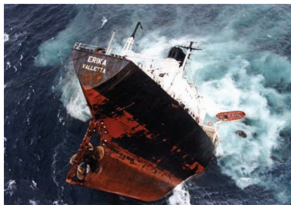
Figure 30 The tanker ERIKA – lost as a result of steel corrosion (BBC News, 1999)
