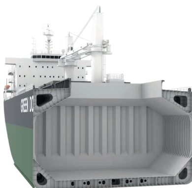
Figure 6 Cross-section of bulk carrier showing cargo space (center) and ballast water tanks (gCaptain, 2019)
