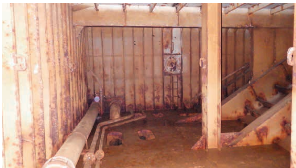
Figure 29 Corrosion of steel in a ballast tank (D. Smith)
